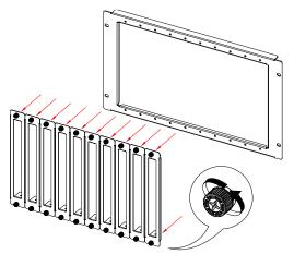
Step 2. Remove the screws from the IP5000 unit's enclosures on two sides.
