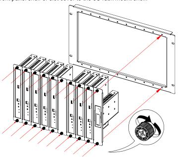
**Step 6.** Install the rack mount shelf on an equipment cabinet using rack screws (not included in the package).
