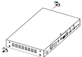
Step 3. Attach the IP5000 unit to the shelf with screws (2 pcs from Step 2, 2 pcs from the package).
